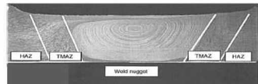
Figure 2: Different micro-structurally distinct regions in FSW
