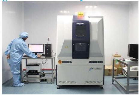
High Resolution X-ray Diffractometer at Center for Nanoscience & Nanotechnology
